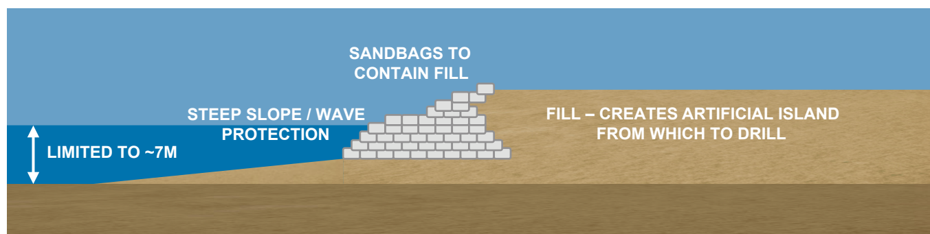
Figure 1-18. Typical Sandbag Retained Island Schematic
